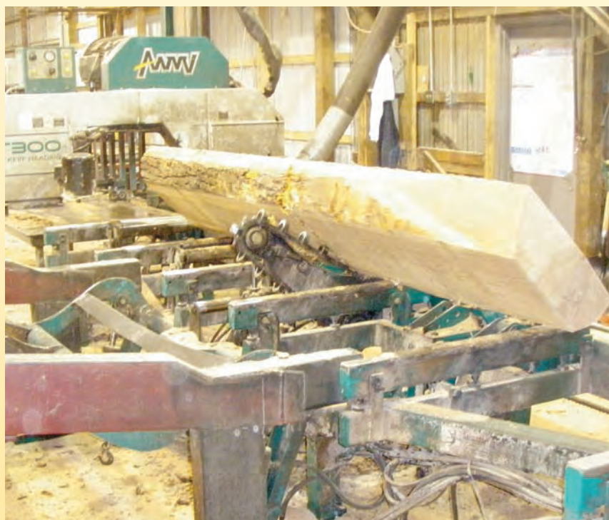
Above: The chain log turner is heavy enough to handle any log that the mill can cut, yet precise enough to position smaller pieces.
