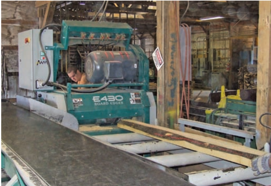
An AWMV E430 Board Edger modified to fit Jennings County Pallets system edges and splits boards off the sawmill to the precise widths required in the pallet assembly operation.
