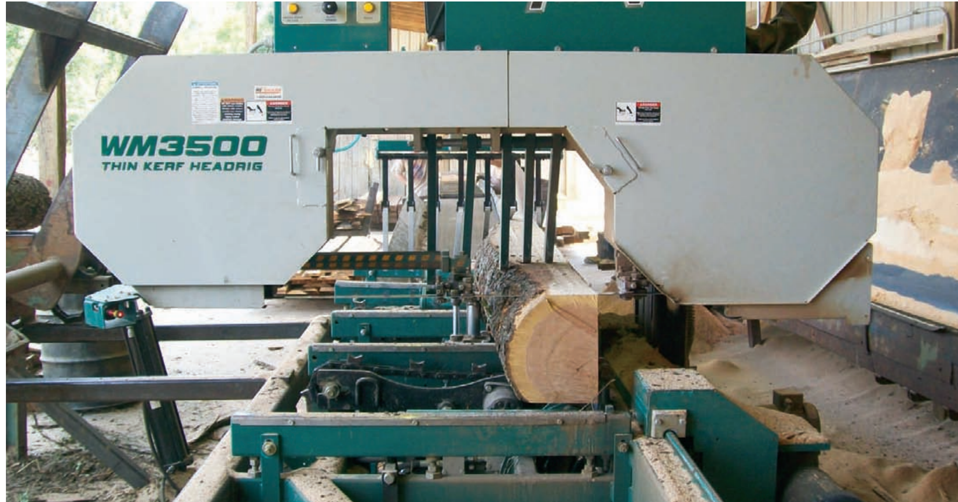
Switching from traditional circle mills to Wood-Mizer's thin-kerf bandsaw mills increased production and log-to-lumber footages.
