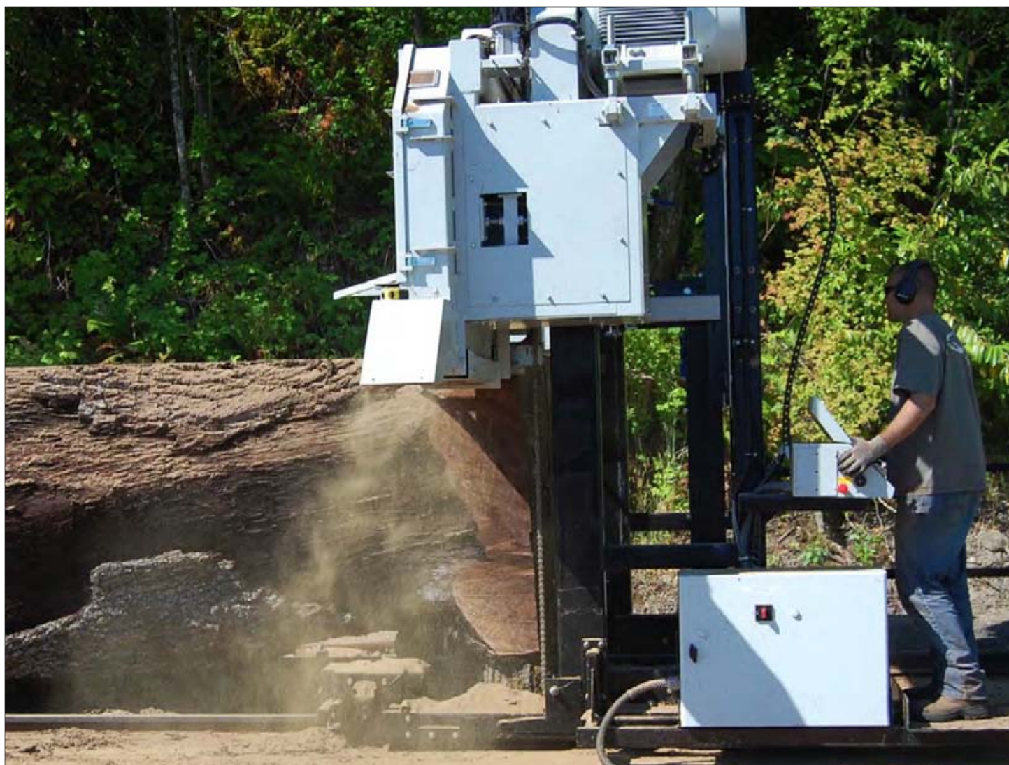
Sawing huge logs with the WM1000 is made easier with the ride-along operator station and computerized networks.
